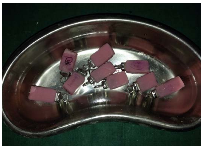
Fig.6: Luted specimens immersed in water
