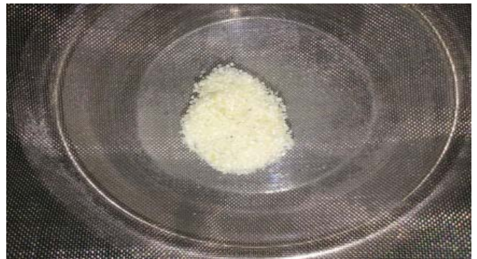
Fig. 8: graft particle passing through 300 \mu\text{m} sieve
