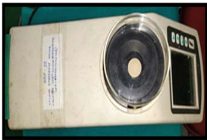
Figure 2: Color measurement using spectrophotometer
