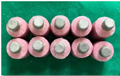
Figure 3: Ni-Cr alloy copings seated on working dies mounted in acrylic base.
