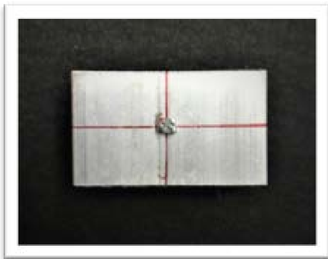
Fig. 1: Jig prepared with bracket bonded
