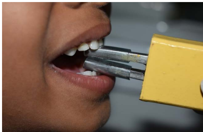
Figure 3: Measuring bite force in anterior region
