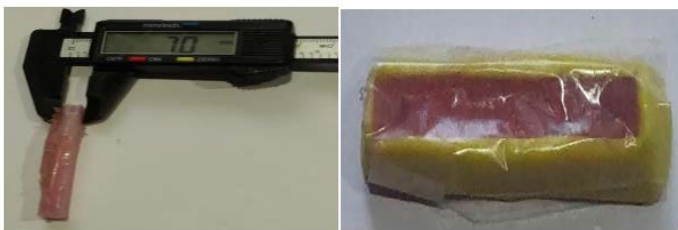
Figure 6: Packing of Soft Liner on surface treated acrylic resin samples
