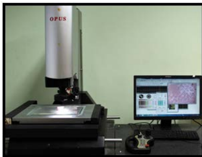
Figure 3: Sample ready for observation in the Visual Measurement Microscope.
