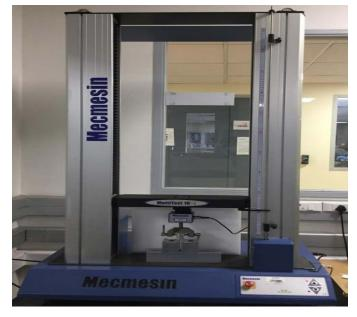
Figure 7: Universal Testing Machine (Mecmesin)
