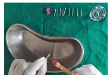
Figure 3: Treatment with 9% hydrofluoric acid. 1.3.4. Etching with 99% Dichloromethane
