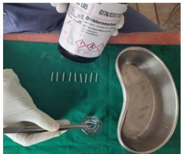
Figure 4: Treatment with 99% Dichloromethane 1.3.5. Evaluation of Surface Roughness – Optical Profilometer
