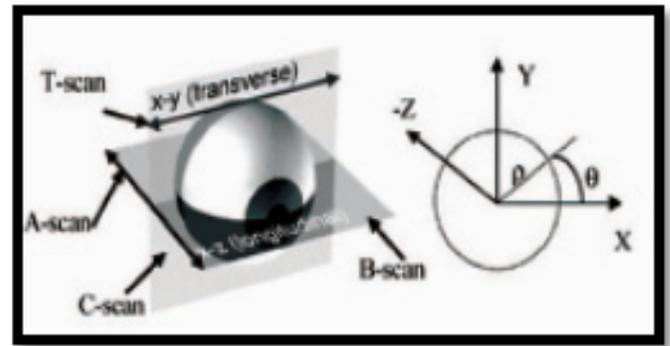
**Figure 4:** Relative orientation of the axial scan (A-scan), longitudinal slice (B-scan), x-y (transverse) scan (T-scan) and en-face or transverse slice (C-scan).
