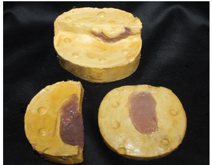
Fig. 10: Packing of the three-piece mold
