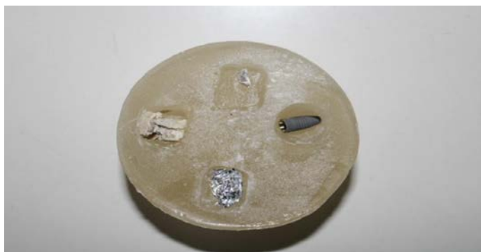
Figure 2: shows the PMMA phantom with materials used for analysis.
