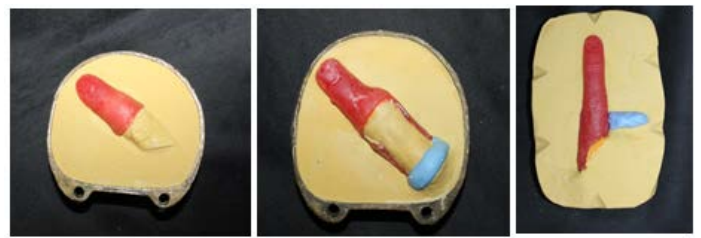
Figure 9: Investing of wax pattern
