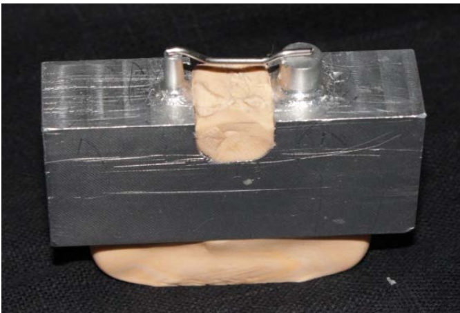
Figure 3: 0.9 mm stainless steel wire stabilised on the occlusal third of the simulated abutment teeth
