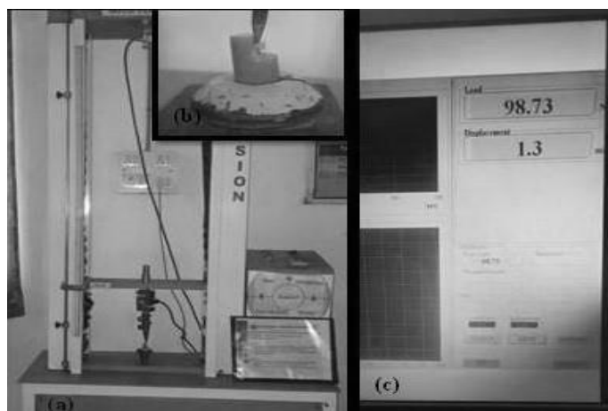
Figure 2: Evaluation of Shear Bond strength in UTM
