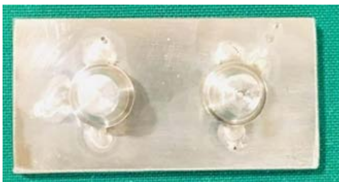
Figure 1 : Master Model Fabricated by using stainless steel dies.
