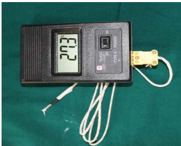
Fig 2: Thermocouple for measuring temperature
