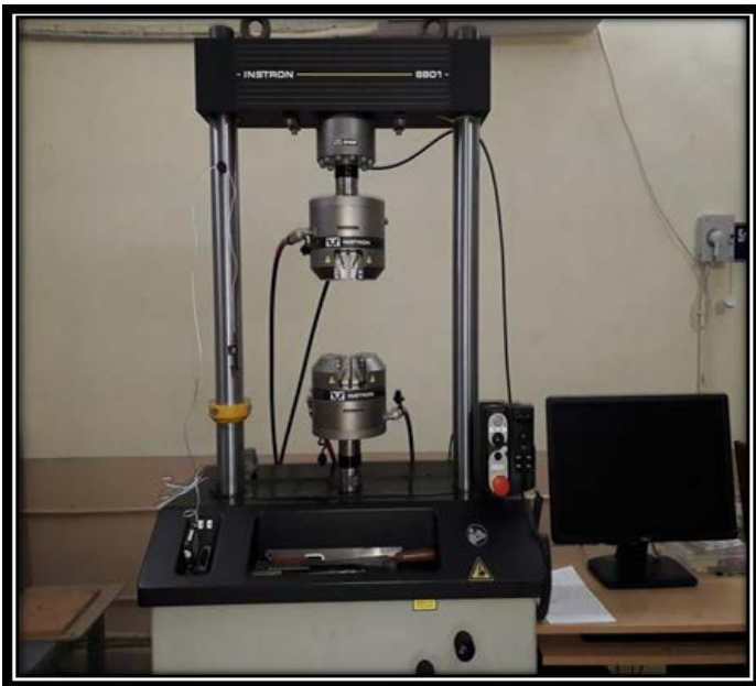
Fig.37: Universal testing machine (instron) 3-point bend test (flexural strength measurements)
