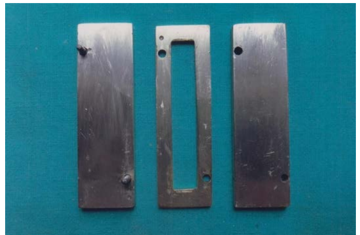
Figure 10: Die for fabrication of specimens for flexural strength testing
