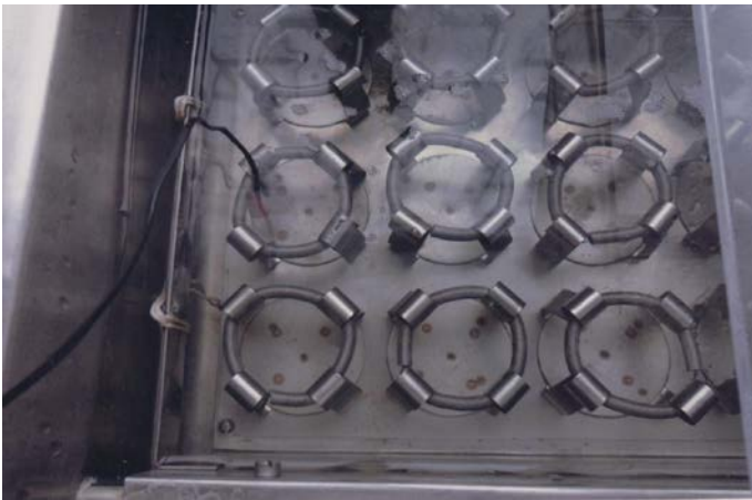
Figure 6: Thermal diffusivity specimen placed in water bath maintained at 70 \pm 1^\circ\text{C}
