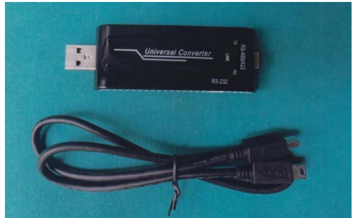
Figure 9: Universal converter KA301(Serial digital converter, TAIE, Taiwan) along with wire which connect it with RS 485
