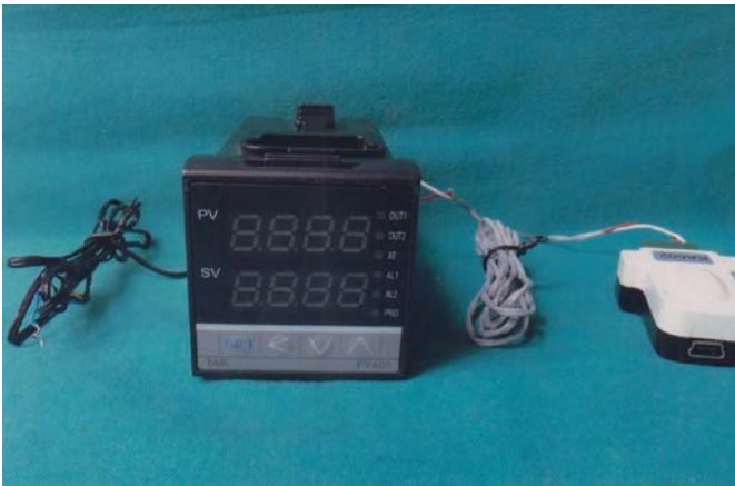
Figure 7: Digital PID Controller (Digital manufacturers, TAIE Taiwan) along with RS-485
