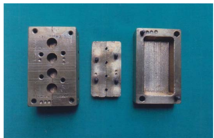
Figure 5: Die for fabrication of thermal diffusivity specimens
