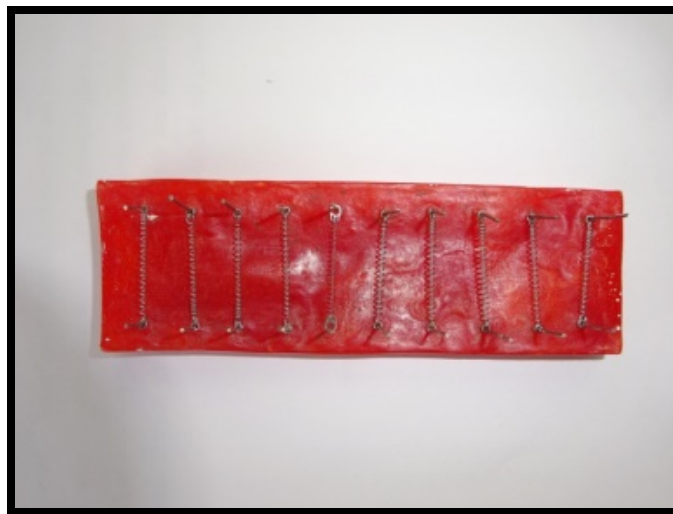
Figure 1: Acrylic jigs with stainless steel pins
