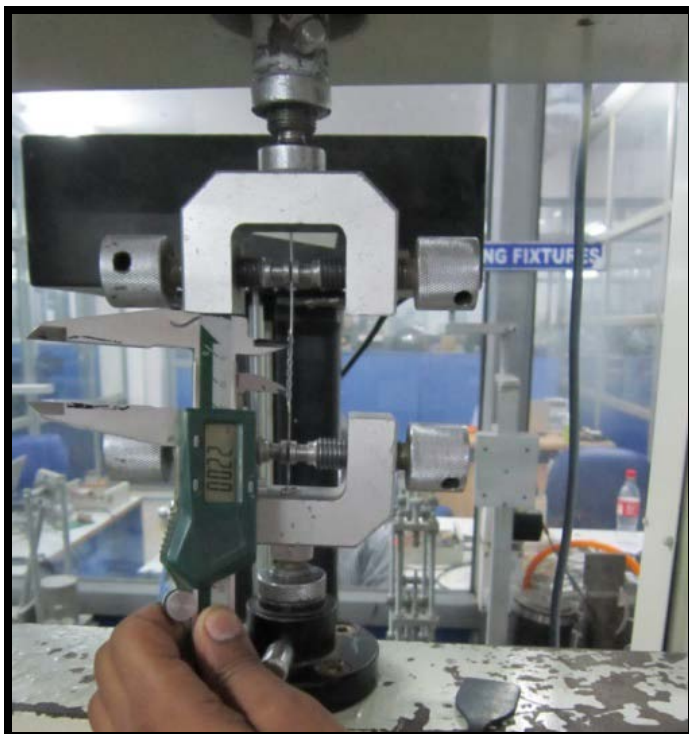
Figure 3: Elastomeric Chains stretched on the vertical jig clamped on the Universal testing machine at 22 mm
