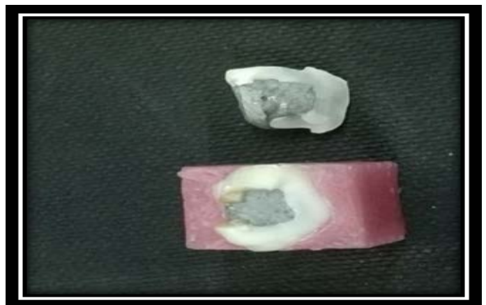
Figure 7: Fracture of the core material
