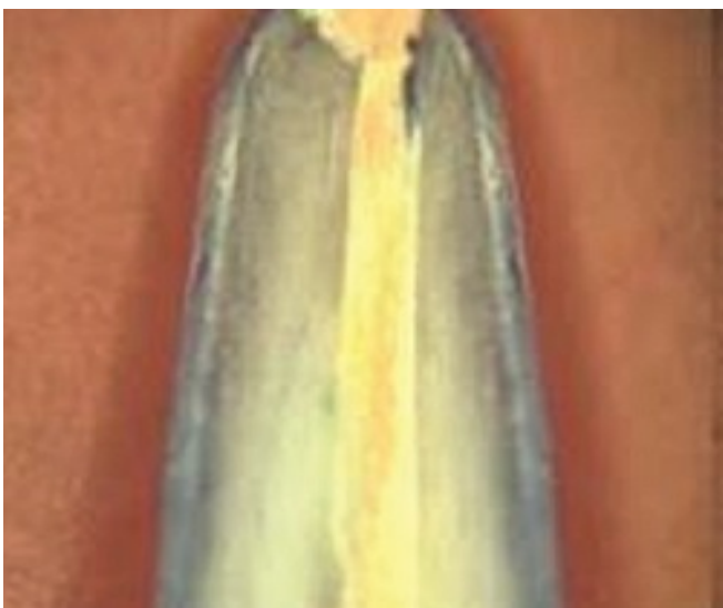
Figure 3: specimen shows dye penetration of BioRoot RCS
