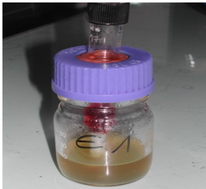
Figure 2. Model System E1 showing two compartments: tube with only vial and flask containing vial inoculated with E. faecalis
