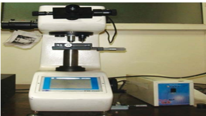
Figure 4: Vickers hardness tester
