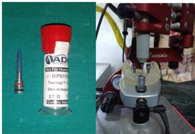
Fig 2: Placing implant replicas with the milling machine
