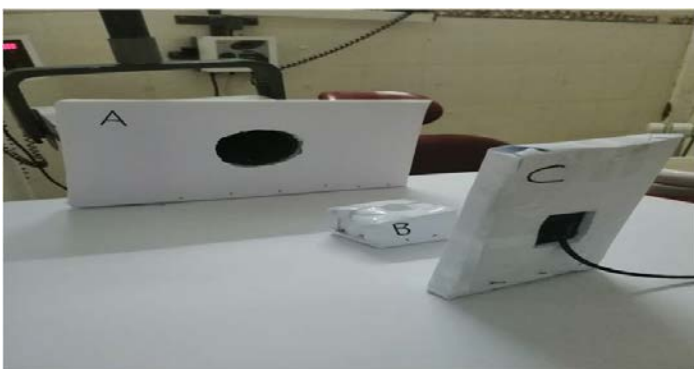
Figure 3: Fixation system. (A) Fixation place of the radiological cone. (B) Fixation place for the tooth sample (C) Fixation place for the radiological sensor
