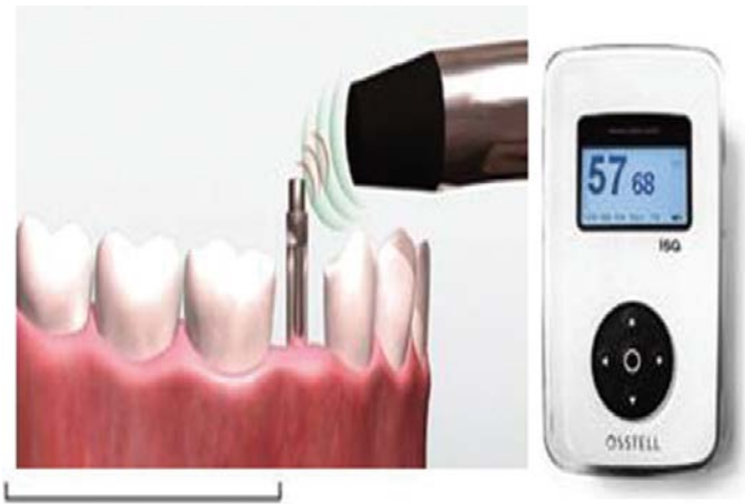
Figure 4: Principle of the Osstell Mentor™. Magnetic peg (smart peg™) works like a tuning fork and Osstell ISQ™ www.osstell.com, April 2011
