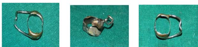
Figure 4(a): Loop fracture Figure 4(b): Solder breakage Figure 4(c): Decementation
