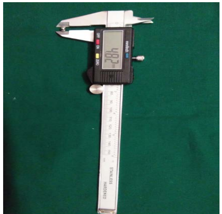
Fig 3: Measurement of metal ball diameter as reference
