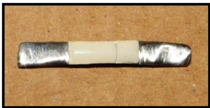
Figure-5: Cohesive failure
