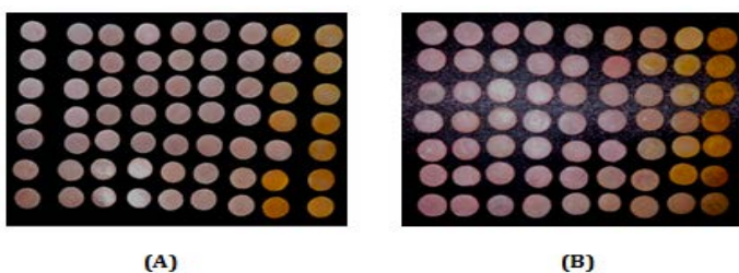
Figure 4: Test samples 63 days after immersion ( \Delta E_3 ): A) High Impact Denture Base Resin B) Flexible Denture Resin
