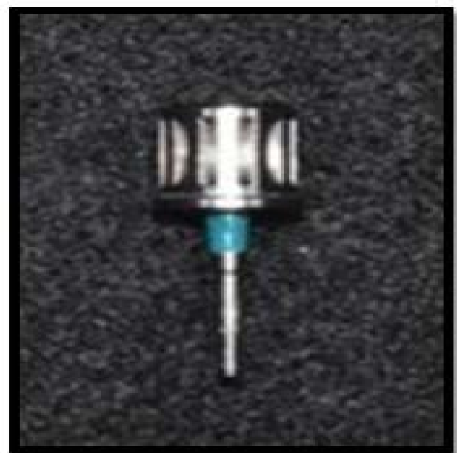
Fig. 9: Removal driver. The tip pushes the top of the abutment, forcing the Zirconia balls against the nitinol spring, thus disengaging the crown.
