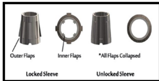
Fig. 3: Occlusal and profile view of the shape memory sleeve demonstrating the locked and unlocked configurations.
