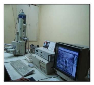
Fig.6: Microstructural analysis using Jeol 35 SEM fitted with the Deben Genie upgrade
