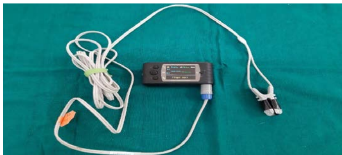
Figure 2- Customized pulse oximeter
