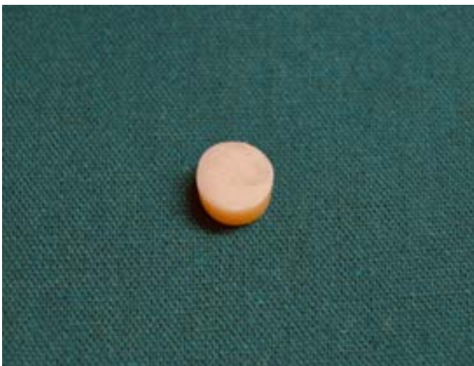
Figure 1: Cylindrical specimen of composite for testing Following polymerization, the specimens were removed from the mould and were polished with Super Snap (Shofu, Inc. Kyoto, Japan) to remove any surface defects
