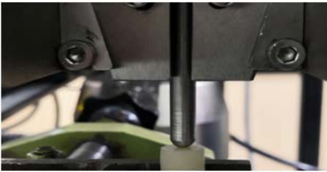
Figure 3 (b): Metallic sphere contacting the specimen surface for cyclic loading
