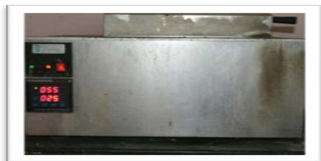
Figure 9: the specimens were thermocycled for 24Hrs. Each cycles consist of 15s of immersion in 15 degree celcius water bath, 10 S Dwell time 15s immersion in 55 degree celcius water bath.
