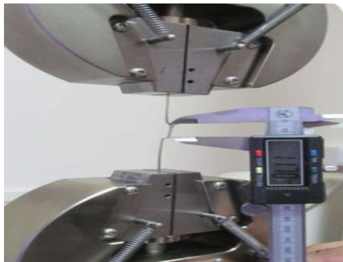
Fig. 3: After Stretching For Measurement. Extension Confirmed By Digital Vernier Caliper
