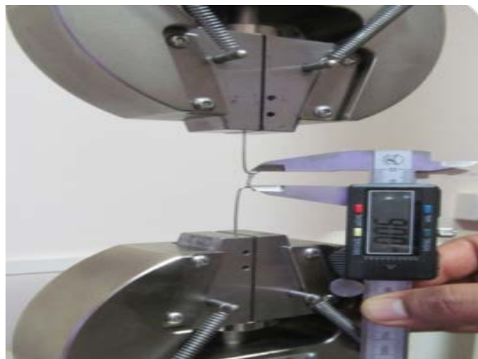
Fig. 2: Coil Spring Placed In Instron Universal Testing Machine –Initial Position
