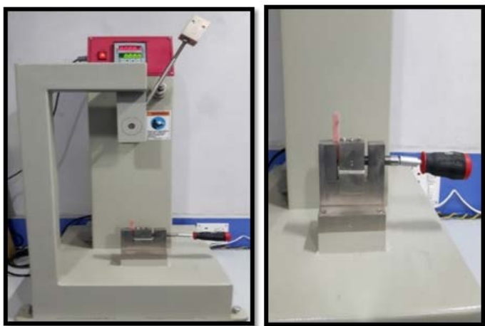
Fig 19: Izod Impact Testing Machine for Izod impact strength test.
