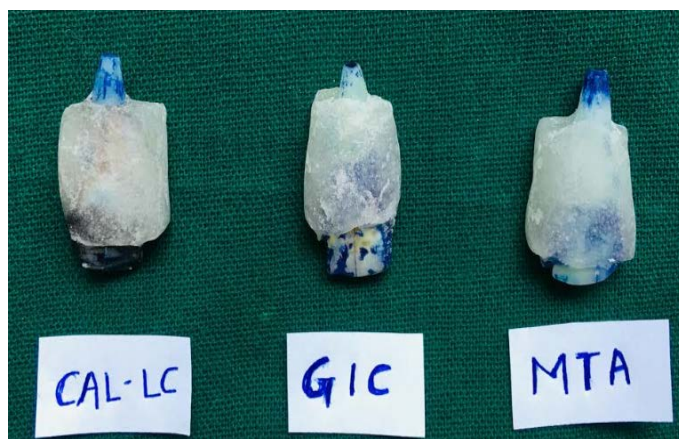
Fig. 8: Clear acrylic blocks made to stabilise teeth during sectioning.
