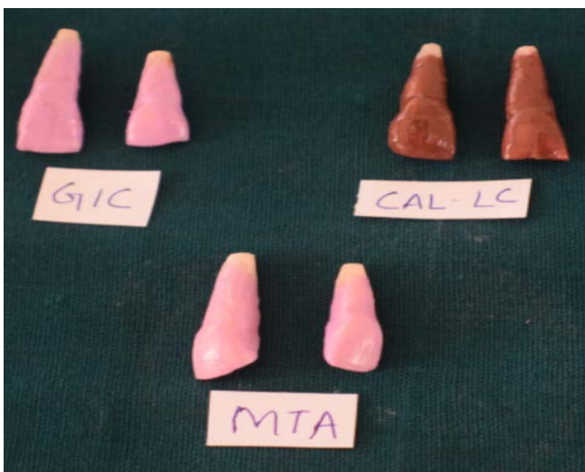
Fig.7: Nail varnish coat except for the apical 1mm
