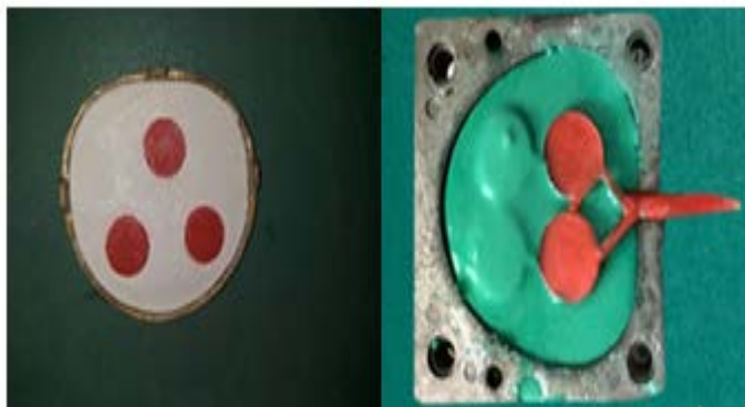
Figure 3: Wax pattern in conventional flask and special flask for injection moulding technique
