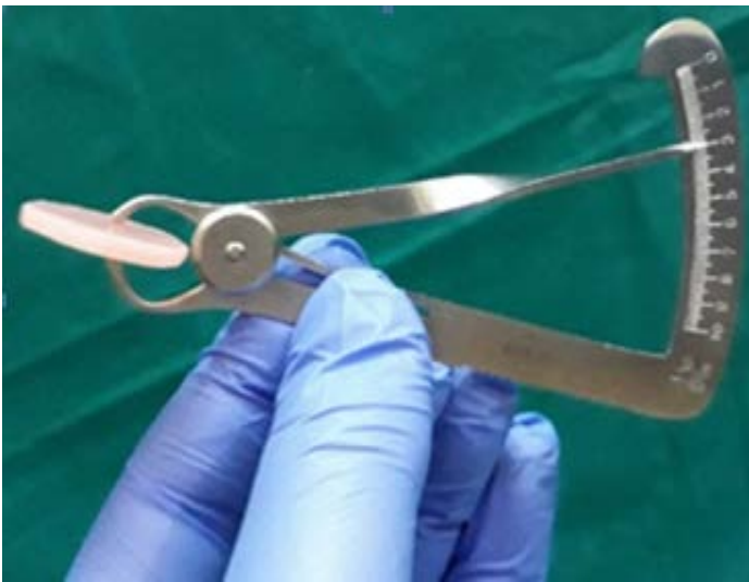
Figure 2b: 3 mm thickness of sample
