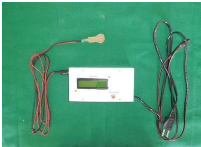
Fig 1: Lip Pressure tester (Flexiforce Sensor and Data analog to Digital converter) Model A301 (Tekscan)
