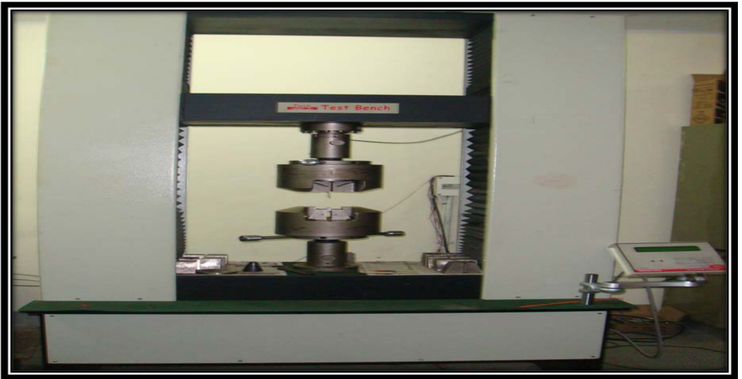
Figure 8: Fracture Strength testing on a mounted specimen
