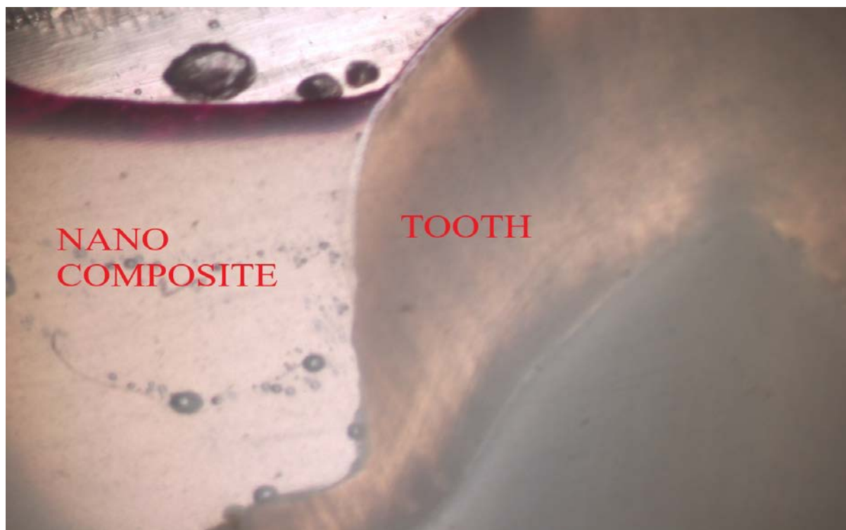
Figure 2: Stereomicroscopic view of Miracle mix under 80X magnification
