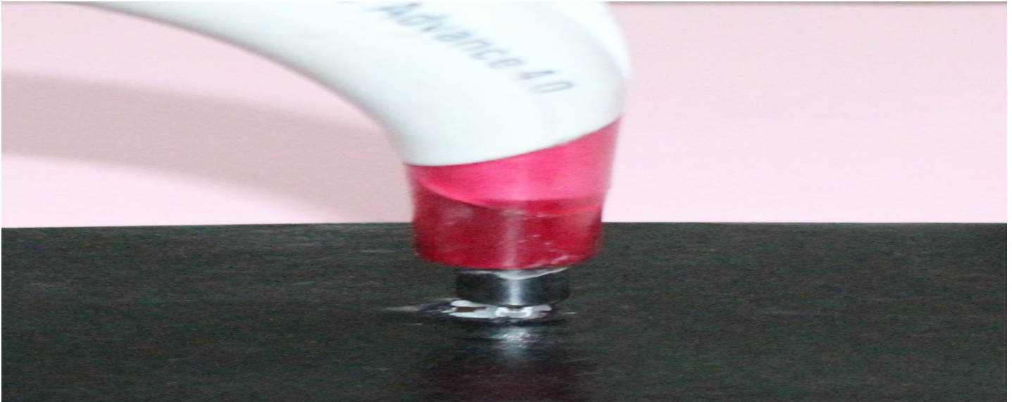
Fig. 1: Spectrophotometer in Position to Read the Colour Parameter L* A* and B* Of Non-Translucent Brackets-In Vitro
