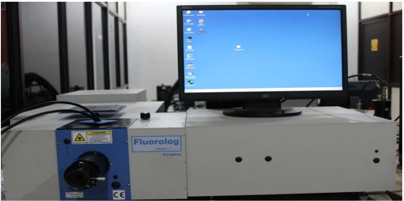
Fig 3: Diffuse Reflectance Spectrometry- To Measure the Percentage (T %) Of Transmittance from the Percentage of Reflectance of All Brackets.
