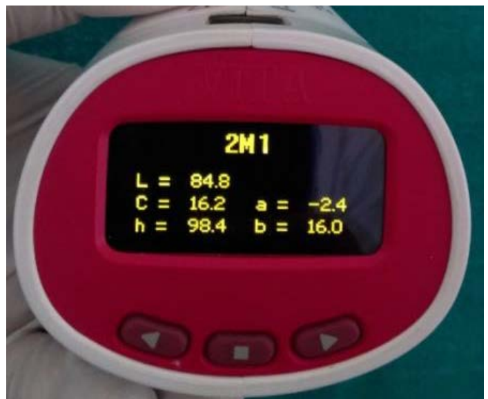
Fig. 11: Color difference metric value as compared to the corresponding Vita 3D master shade guide
