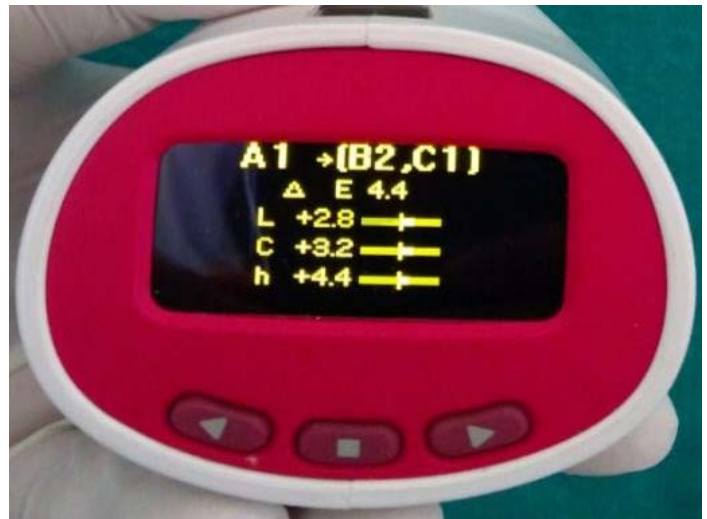
Fig.10: Color difference metric values as Compared to the corresponding Vita Classic shade guide
