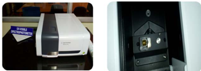
Figure 3: A-UV-Visible Spectrophotometer and B- Disinfectant placed in cuvette.
