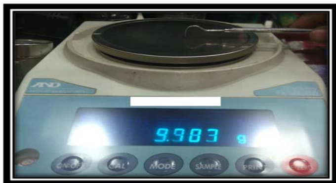
Fig 1: Measurement of tactile force by digital balance
