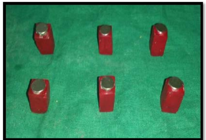
Figure 3-Neodymium Iron Boron magnets mounted on acrylic block
