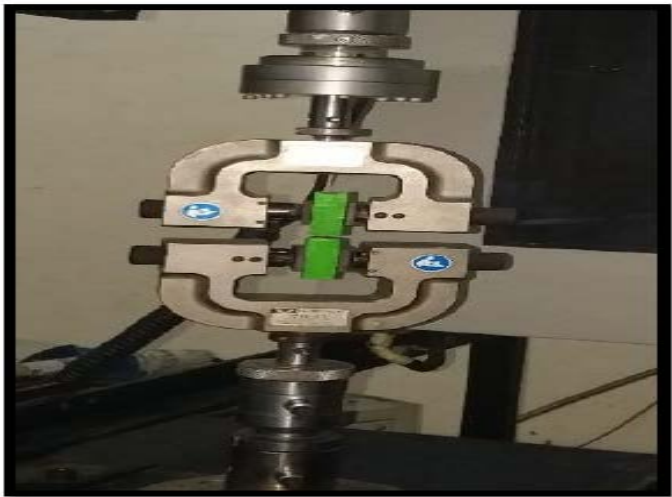
Figure 5: Samarium Cobalt magnets mounted on Instron Universal testing machine for testing
