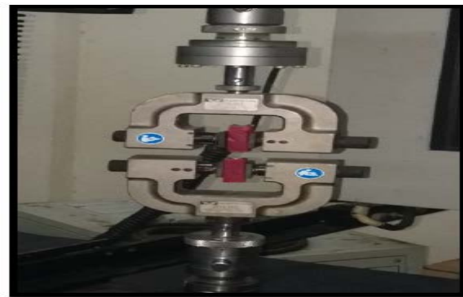
Figure 6: Neodymium Iron Boron magnets mounted on Instron Universal testing machine
