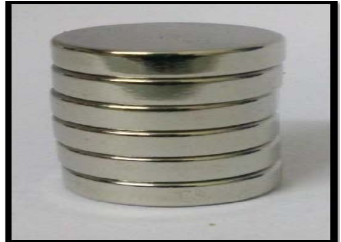
Figure 1: Neodymium Iron Boron magnets used for the study
