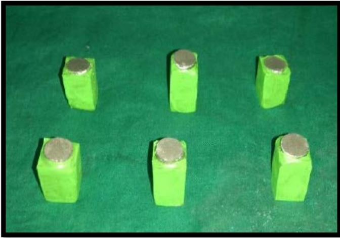
Figure 4- Samarium Cobalt magnets mounted on acrylic block
