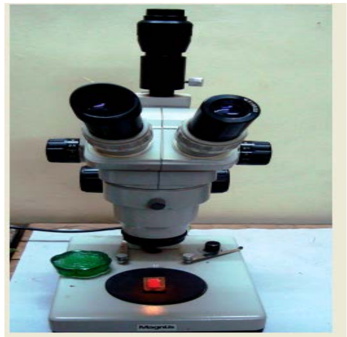
Figure 7: Stereomicroscope used to measure cement spaces.
