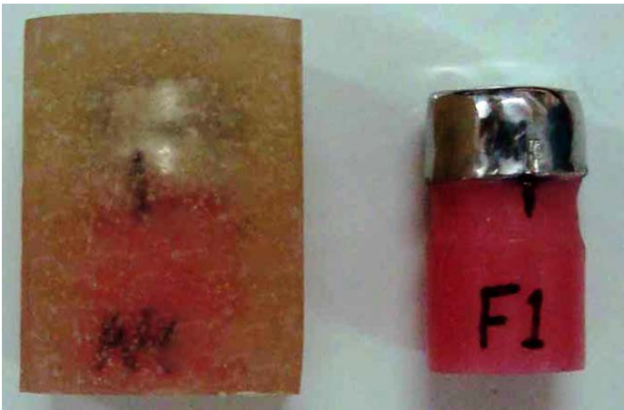
Figure 5: Crown-die assembly embedded in clear acrylic.
