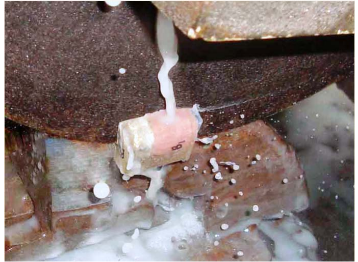
Figure 6: Sectioning of embedded crown-die assembly with Carbide disc using water with added detergent as a coolant.
