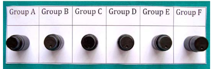
Figure 1b: Metal dies of six finish line preparations machined on computerized numerical control (CNC) machine.
