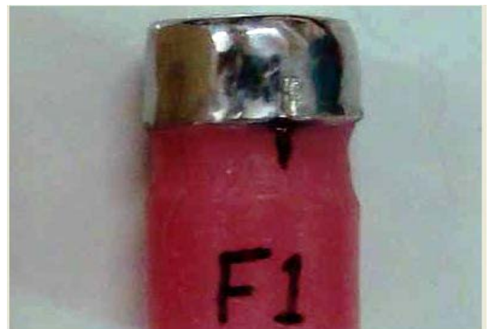
Figure 3: Dies were indexed to aid proper repositioning during cementation by drawing a vertical line on the acrylic below the vertical groove of metal crown.
