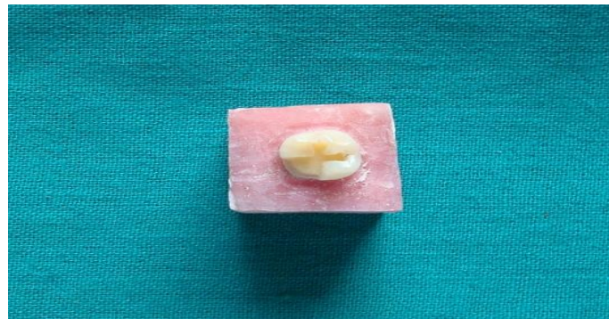
Fig. 3: Specimen Mounted With Acrylic Block
